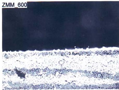
Figure 7 (c) SEM image of LaMnO<sub>3</sub> film thickness at 500° C
