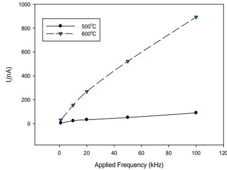
Figure 8 (d) The variation of current loss with different frequencies
