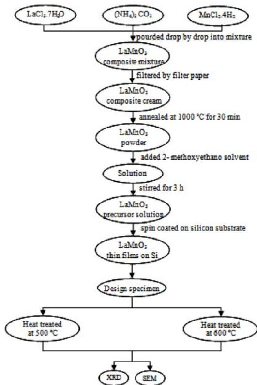
Figure 1 Flow chat for preparation of LnMnO<sub>3</sub> thin films
