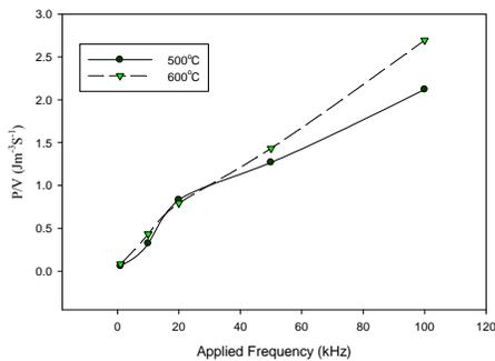
Figure 8 (e) The variation of power dissipation with different frequencies
