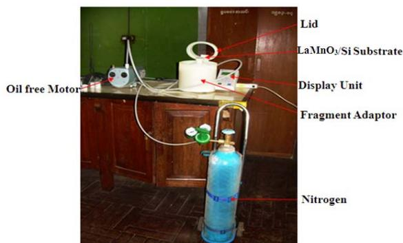
Figure 3 The photograph of spin coating system of the spin processor (MODEL WS-400BZ- 6N PP/LITE)
