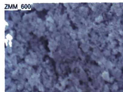
Figure 7 (b) SEM image of LaMnO<sub>3</sub> thin film at 600° C
