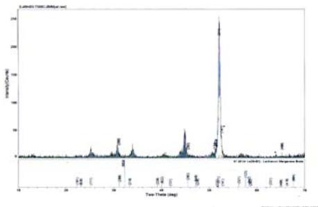
Figure 5 (b) XRD profile of LMO<sub>3</sub> thin film at annealing temperature
