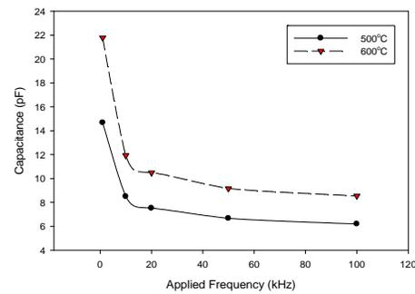
Figure 8 (a) The variation of capacitance with different frequencies
