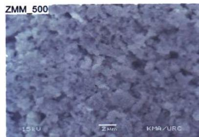
Figure 7 (a) SEM image of LaMnO<sub>3</sub> thin film at 500° C
