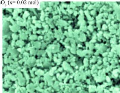
Figure 6 SEM image of LaMnO<sub>3</sub> powder at 1000° C
