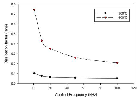
Figure 8 (b) The variation of dissipation factor with different frequencies
